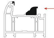
Fit a 17mm Frame Wedge to the outer frame on the stay fixing area
