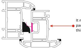
It may be necessary to pack the sash/glass at this point as shown
