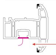
Fit a Sash Spring to the sash on the center line of the stay fixing area
